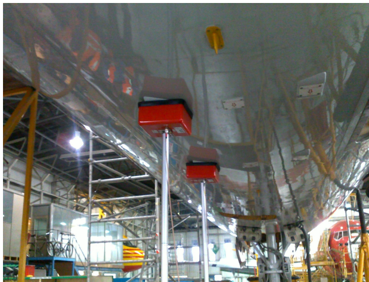
Fig. 4-12 ALT-8000 Antenna Coupler Installed
