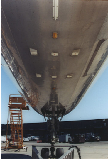
Fig. 6-7 Triple LRRRA Antenna Installation (ARINC square patch type)
