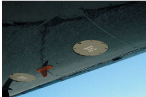
Fig. 6-8 LRRRA Antenna Installation (recessed horn type)
